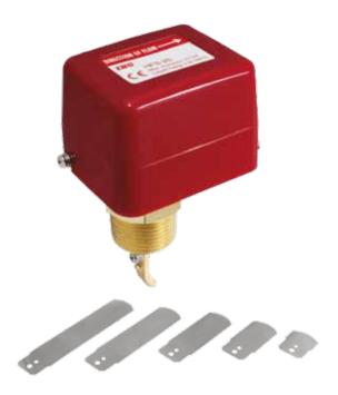
UNIQUE Water Flow Switch is used to monitor the start-stop flow of water in the system. For the sprinkler system to work optimally, there must be sufficient water flow. The switch is also used to shut equipment down to prevent damage to the system if the water flow drops to a pre-determined rate. The switch fits 1" NPT connections.
