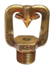
Use HD's non-automatic Medium Velocity (MV) water spray nozzles in deluge water spray systems to give special hazard fire protection. Small droplets of water are discharged via an external deflector in a solid cone shaped pattern that uniformly covers the surfaces to be protected. This action cools the surfaces (whether vertical, horizontal, curved or irregular), prevents excessive heat absorption from fire and averts structural damage or spread of fire.
